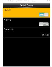
**RS232:** Whether to use RS232 to communicate with PC. **RS485**: Whether to use RS485 to communicate with PC.
