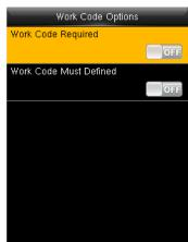
**Work Code Required**: The work code must be input during verification. Select whether to enable this function. **Work Code Must Defined**: The input work code has to exist
