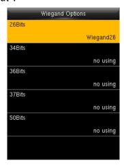
**Wiegand Format**: The system has five built-in formats: Wiegand 26-bits, Wiegand 34-bits, Wiegand 37-bits and Wiegand 50-bits. Every format has two types of WiegandX and WiegandXa except for Wiegand 50-bits. You can select more than one wiegand formats.
